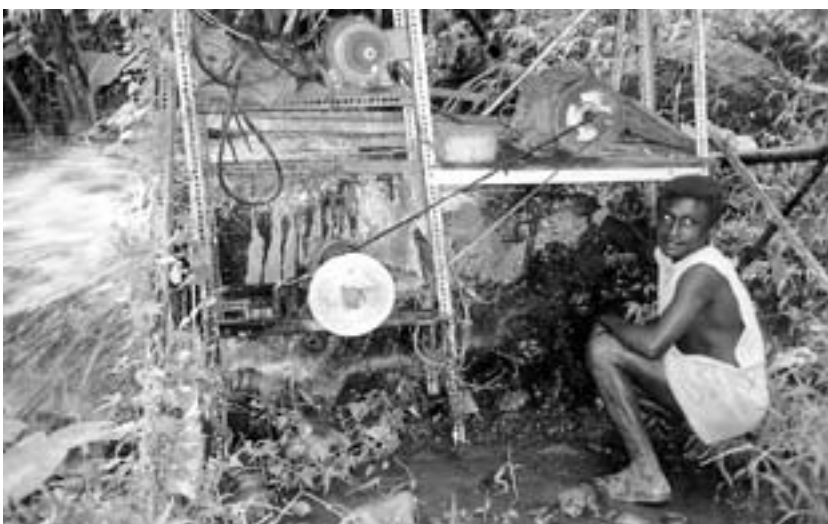
A micro-hydroelectric turbine typical of those made from scavenged parts during the civil war.
